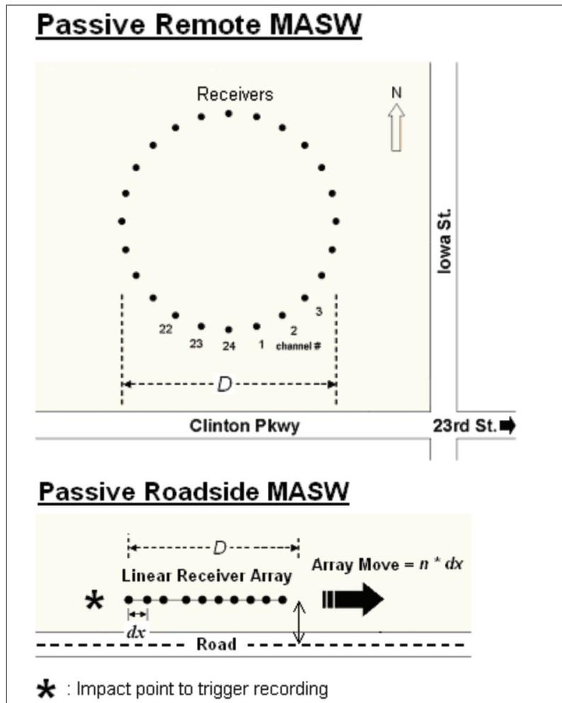
Figure 3. Schematics of data acquisition with passive remote and passive roadside MASW.
