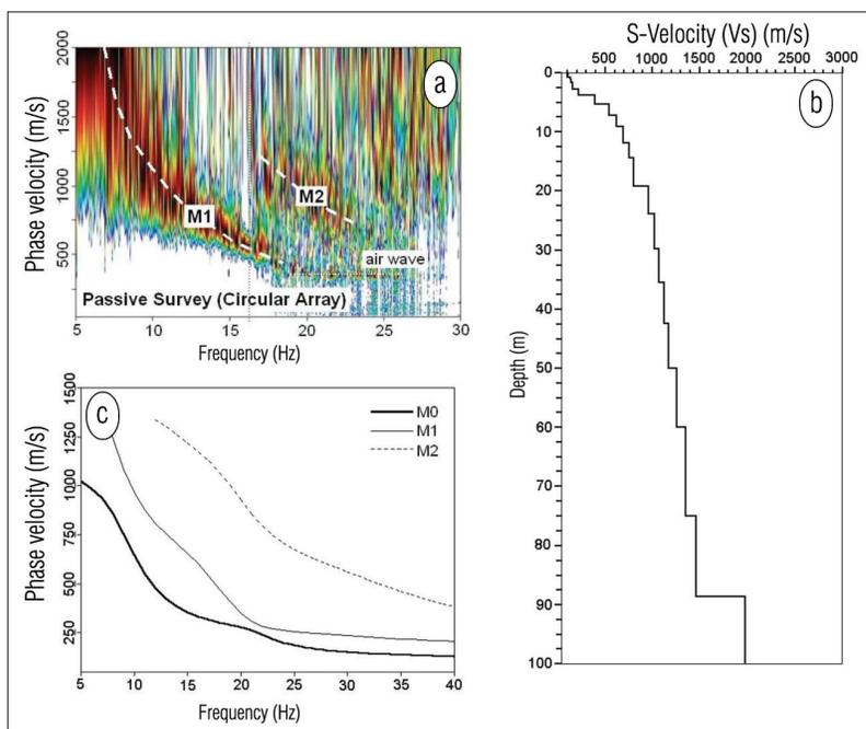
**Figure 4.** (a) Dispersion image obtained from a passive remote MASW survey using a circular receiver of 115-m diameter. (b) 1D  $V_S$  profile inverted from the two dispersion trends interpreted in (a). (c) Theoretical dispersion curves calculated from the  $V_S$  model in (b).
