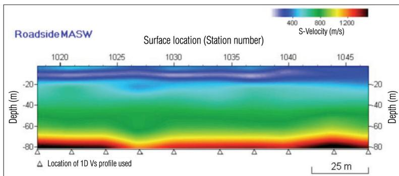
**Figure 5.** 2D  $V_S$  map obtained from a passive roadside MASW survey using a linear 24-channel receiver array of 5-m separation. A sledge hammer delivered impact at one end of the array to trigger 30-s recording. This 2D  $V_S$  map was obtained from a combined analysis of active (0–2 s) and passive (2–30 s) portions of each record.
