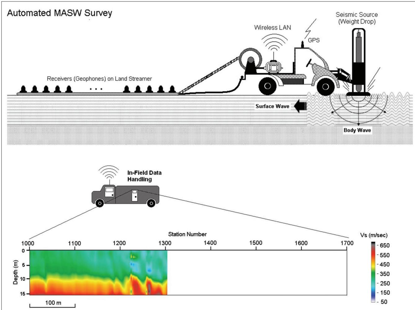
Figure 7. Schematic of a prototype field system recently developed and tested at KGS illustrating the mobility and effectiveness of the routine MASW survey in the near future.
