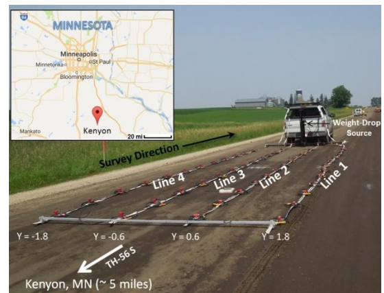
Figure 1. Location map and quadruple land streamers used to acquire MASW data at a test site near Kenyon, MN.
